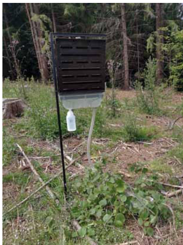
Obrázok 5 a 6. Lapač s hadicou zvedenou ku smrekovému klátu a kláty umiestnené v poraste Figure 5 and 6. Trap with a hose leading to the spruce log, and logs placed in the stand.
